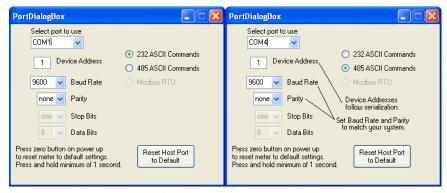
If your unit is RS-485, you'll want to match the Device Address, Baud Rate and Parity to that of your instrument (default settings are shown below). Once you have established communication, you can change the Device Address, Baud Rate, and Parity to set up the instrument for use on your RS-485 Bus system.
