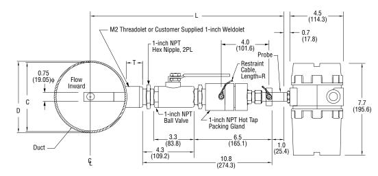
All dimensions are inches. Millimeters are in parentheses. All drawings have a +/-.25-inch (6.4 mm) tolerance. Certified drawings are available on request.
